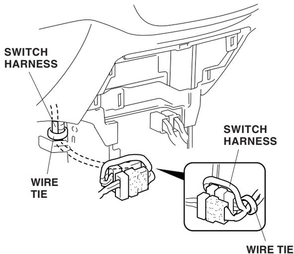
52. Plug the subharness 1-pin connector (routed in step 43) into the switch harness 1-pin connector (blue/red), then wrap one cushion tape around the connectors. Secure the connector to the vehicle harness using one wire tie.
