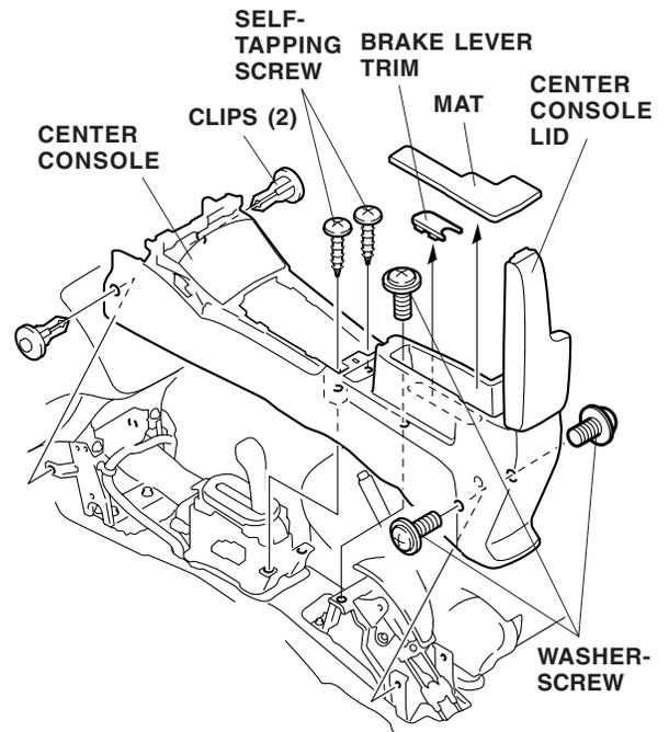
40. Remove the brake lever trim and remove the center console (two self-tapping screws, three washer-screws and two clips).
