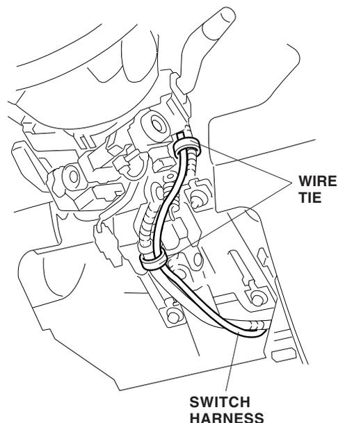
62. Under the dash, secure the switch harness to the vehicle harness with six wire ties in the areas shown.
