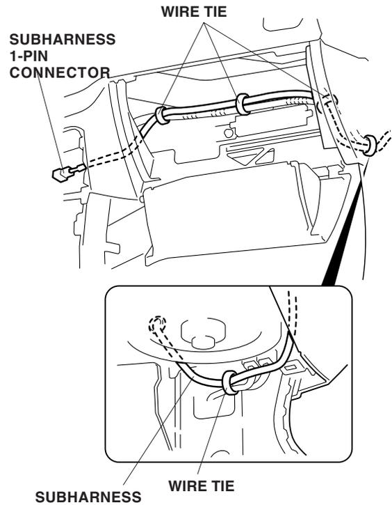
44. Get the switch harness. Route the switch harness under the dash, and over the steering shaft and brake position switch harness.
