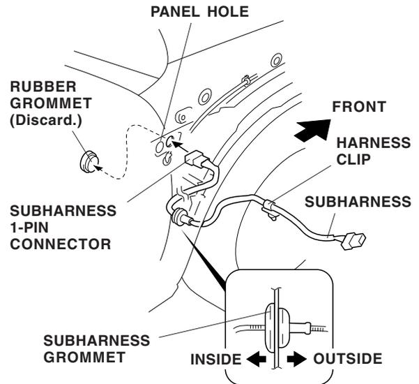
28. Route other end of the subharness through the inner fender toward the front of the vehicle. Plug the subharness 1-pin connector into the fog light harness 1-pin connector routed in step 14.
