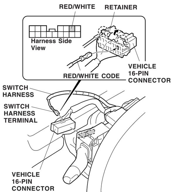
60. Reconnect the vehicle 16-pin connector.
