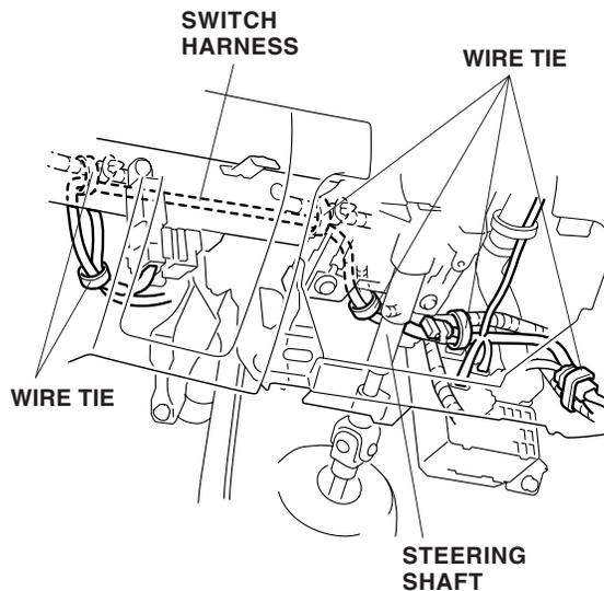
63. Check that all wire harnesses are routed properly and all connectors are plugged in.
