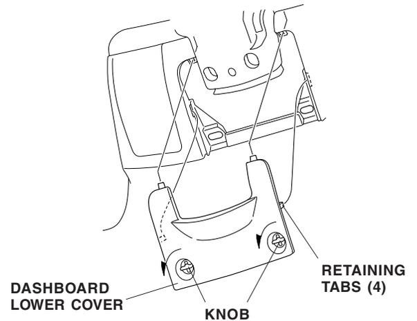
33. Turn the knob counterclockwise, and release the two clips and remove the driver's dashboard under cover.
