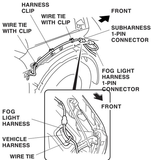
29. Near the 1-pin connector, secure the fog light harness to the vehicle harness with one wire tie in the area shown. Attach the subharness to the inner fender panel with two additional wire ties with clips from the kit, and the one harness clip already attached to the subharness. Insert the clips into the empty holes in the inner fender panel.
