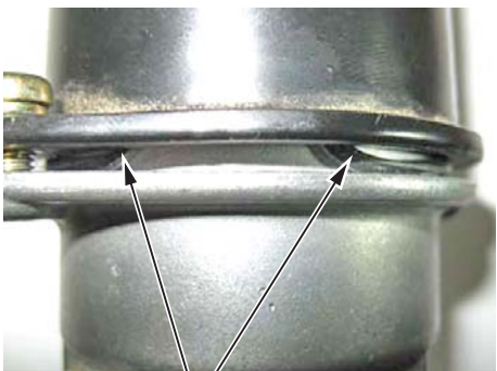
NO GOOD O-ring is pinched and/or rolled.
