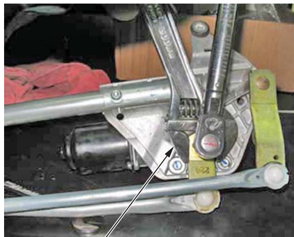
Hold the link while you tighten the nut. 31 N·m (23 lb-ft)
