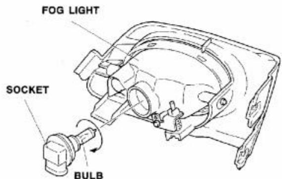
5. Reinstall the fog light in the reverse order of removal.
