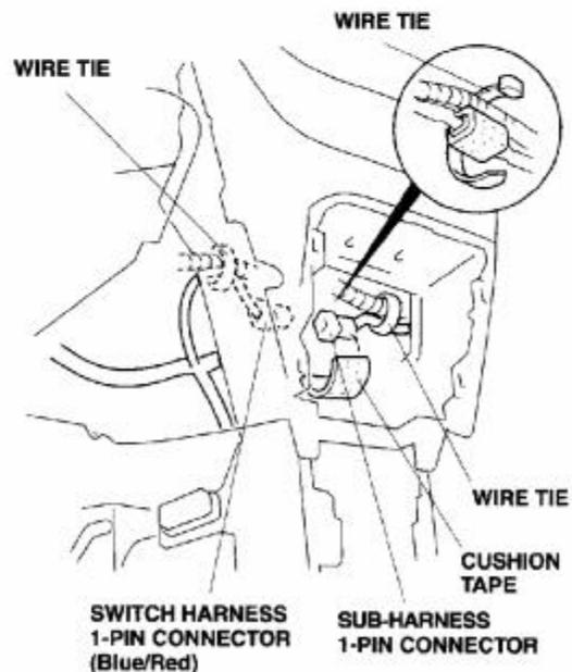
50. Secure the sub-harness and switch harness to the vehicle harness with two wire ties in the areas shown.
