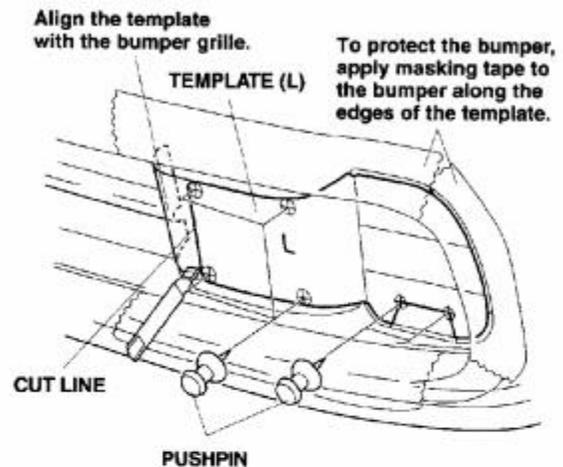
5. Using a pushpin, mark the bumper at each of the six holes indicated on the template.
