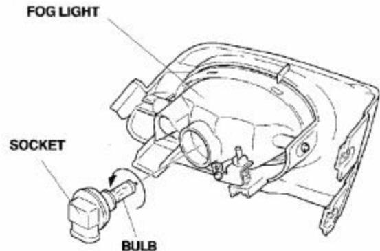
4. Install the new bulb and socket into the fog light.
