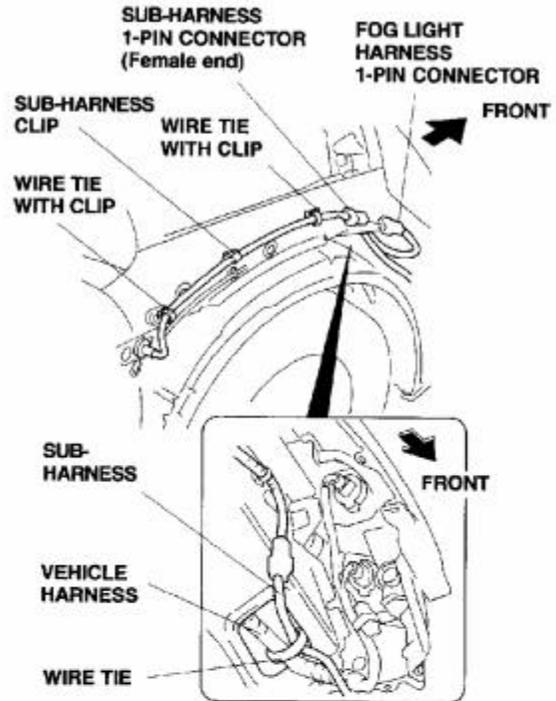
30. Secure the fog light harness to the vehicle harness with one wire tie in the area shown. Secure the sub-harness to the inner fender panel with two wire tie with clips from the kit, and with the one wire tie with clip attached to the sub-harness. Insert the clips into the empty holes in the inner fender panel.
