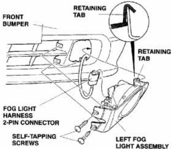
26. Reinstall the left fog light assembly in the front bumper. While holding pressure on the fog light assembly, install the two self-tapping screws to secure the fog light assembly.
