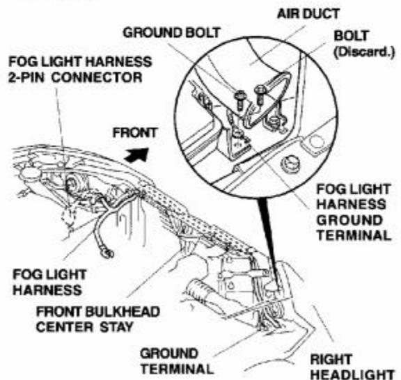
14. Route the other end of the fog light harness toward the driver's side of the vehicle along the vehicle harness, behind the front bulkhead center stay. If the vehicle is not equipped with A/C, the vehicle harness will end at the middle of the vehicle.
