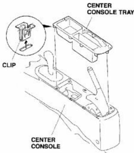
37. Remove the center console (two self-tapping screws, two washer-screws, and two clips). On M/T model, remove the shift knob.
