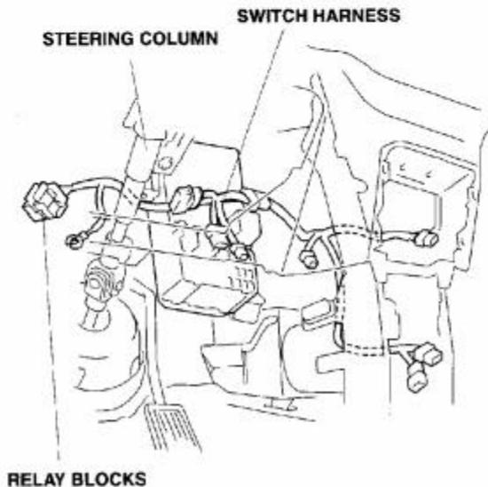
41. Attach the relay bracket to the steering column bracket using the 6 x 16 mm washer-bolt.
