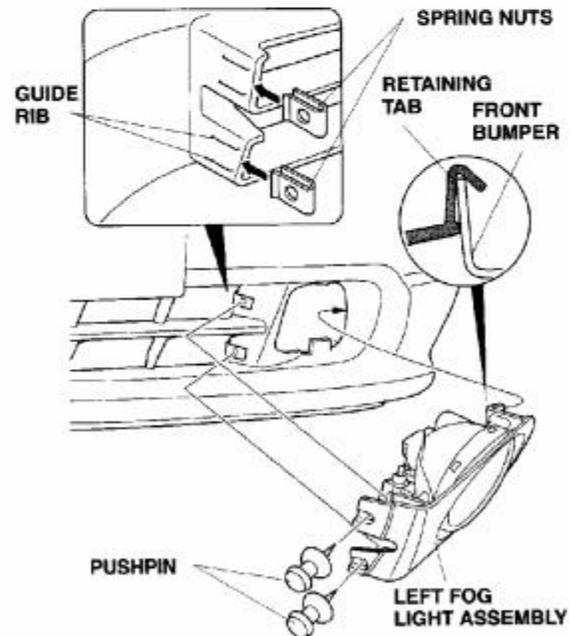
24. Fit the fog light assembly into position in the opening of the front bumper with the retaining tab behind the bumper. Using a pushpin, mark the bumper at each of the two mounting holes, then remove the fog light assembly.
