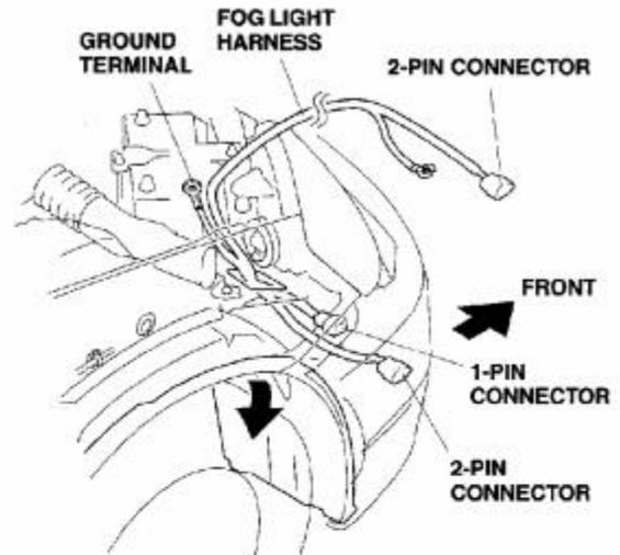
13. Behind the right headlight, remove and discard the bolt that fastens the fuse box bracket. Attach the fog light harness ground terminal and reinstall the fuse box bracket with a ground bolt from the kit.
