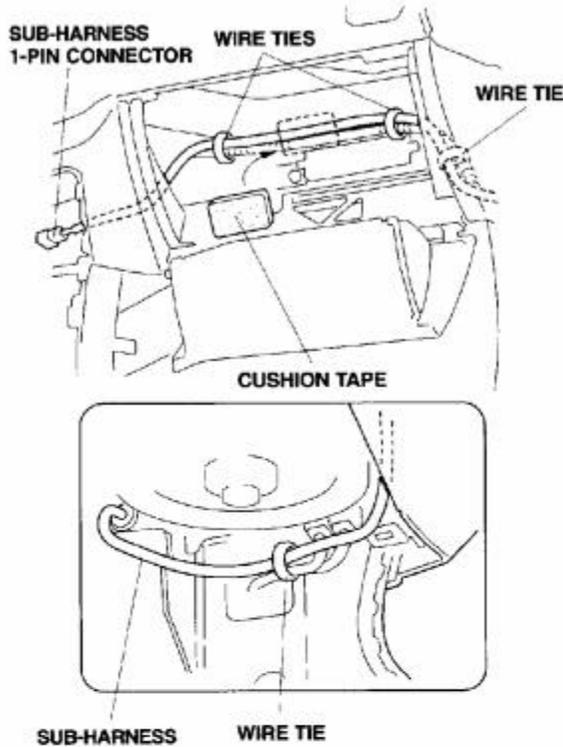
40. Get the switch harness. Route the switch harness under the dash, and over the steering column and the brake position switch harness.
