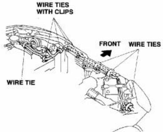
19. On the right (passenger's) side of the vehicle, secure the fog light harness to the hole in the front wheelhouse and to the hole in the front lower cross member, with one wire tie with clip at each location. Do not secure the fog light harness to the yellow SRS harness.
