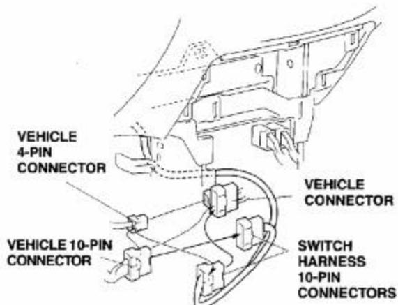
48. Secure the switch harness 10-pin connectors to the vehicle harness 10-pin connectors with one cushion tape. Secure the switch harness to the vehicle harness with two wire ties in the areas shown.
