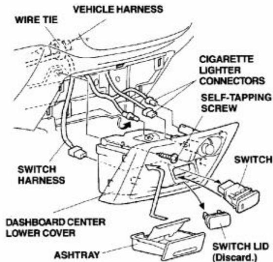
52. Plug the switch harness 5-pin connector into the fog light switch, then install the fog light switch into the dashboard center lower cover.
