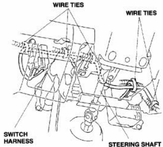
56. Check that all wire harnesses are routed properly and all connectors are plugged in.
