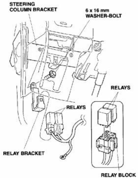
42. Plug the relays into the relay block, then attach the block to the relay bracket.
